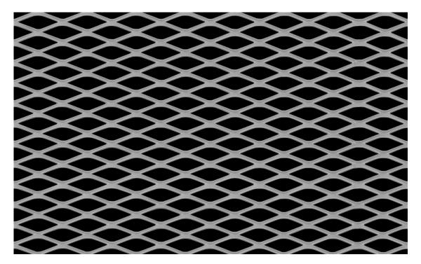
LW Pitch:19.05mmStrand Width:1.71mmSW Pitch:7.26mmThickness:0.70mmWeight:2.70 kg / m2Open Area:53%
